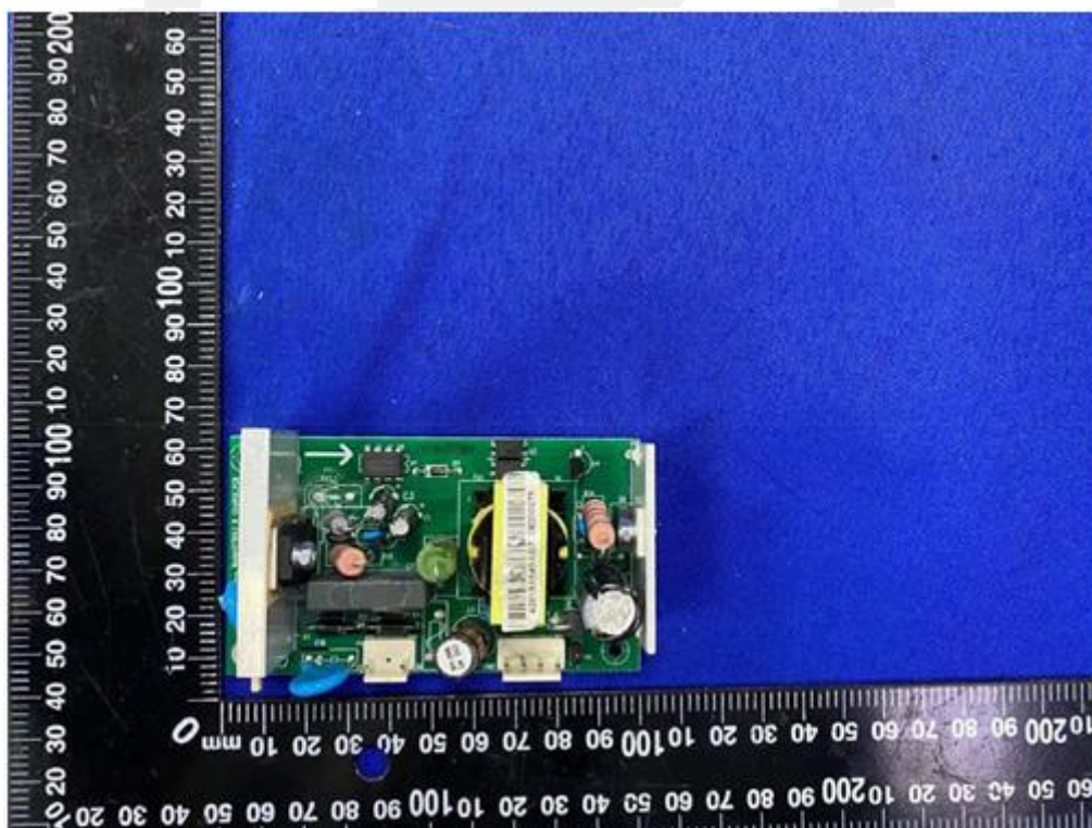
Figure 6: Component side of PCB(3K)
