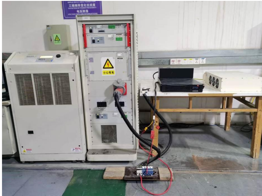
17.10.Photo of Voltage Dips and Interruption Immunity Test
