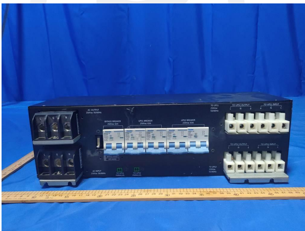
Figure 10: External view of PDU
