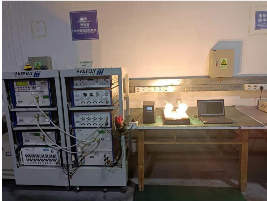
17.8.Photo of Injected Currents Susceptibility Test
