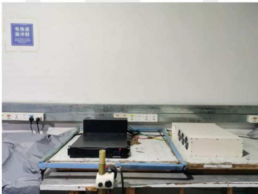
17.9.Photo of Magnetic Field Susceptibility Test
