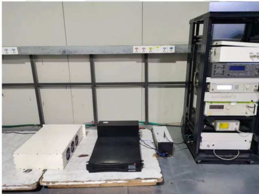
17.8.Photo of Injected Currents Susceptibility Test
