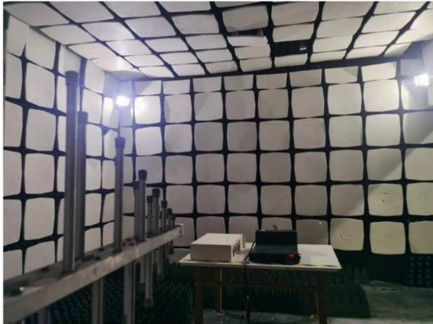
17.5.Photo of RF Field Strength Susceptibility Test
