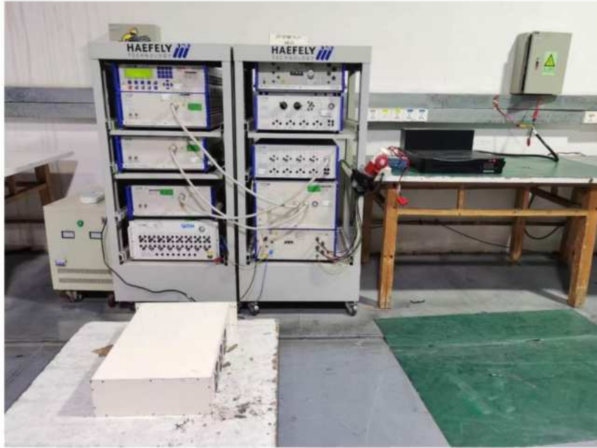
17.8.Photo of Injected Currents Susceptibility Test
